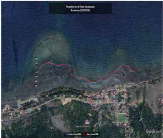
Figure 21. Results of GENESIS Software Simulation Using Breakwater Buildings on Changes in the Karampuana Coastline in 2025 – 2035.
