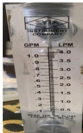
Figure (10.1): Flowrate meter
