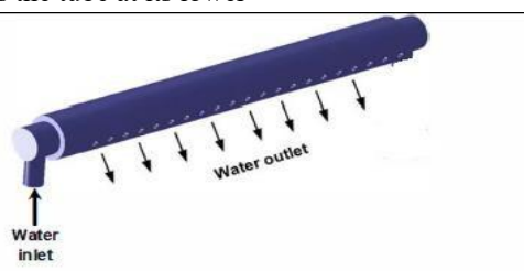
Figure (9.2): perforated supply pipe
