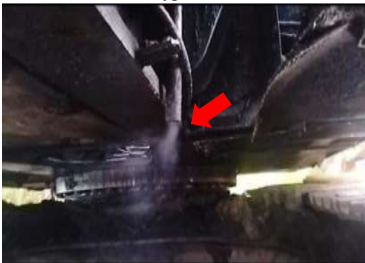
Figure 4. Engine high blowby.
