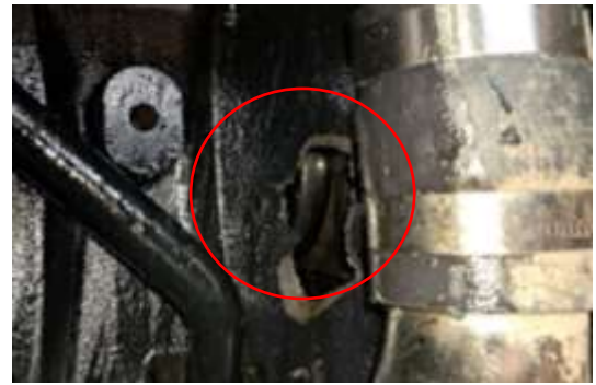
Figure 11. Cylinder block damage.
