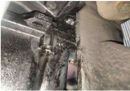
Figure 8. Oil seal leak (Engine Leaking).
