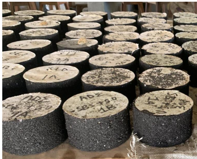
Plate 2. Samples of produced HDPE modified Bituminous Concrete
