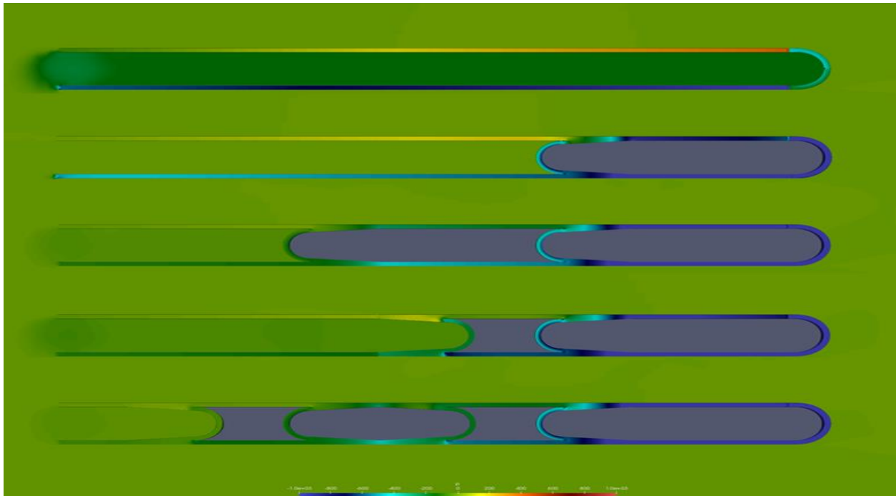
Figure 4. Comparison of pressure profiles (from -1000 to 1000 m 2 /s 2 ) for four configurations of tubes connecting adjacent tunnel entrances and exits. From top to bottom: a) control, b) single recirculation tube, c) two recirculation tubes in series, d) a recirculation paired with a- entrance-exit tube, and e) two pairs recirculation with entrance-exit tubes.
