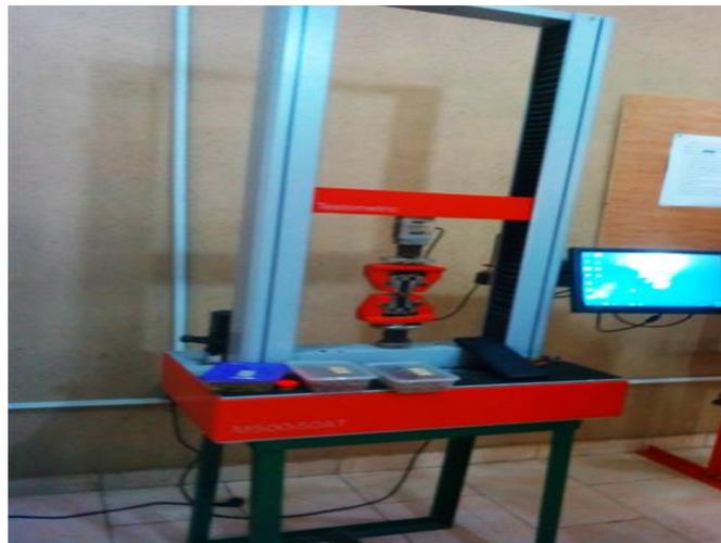
Fig. 9: Compressive test on dried STSM using Universal testometric
