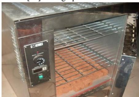
**Fig. 5: Drying of STSM A and B at 200 °C**
