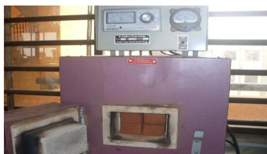
**Fig. 6: Firing of STSM A and B at 700 -1100 °C**
