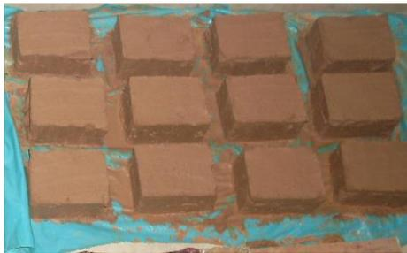
**Fig.3: Moulded STSM A**
