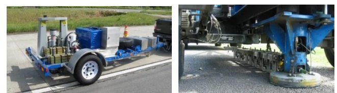
Figure 5. Falling Weight Deflectometer tools
