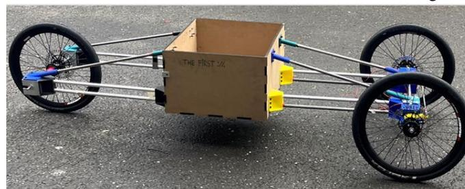
**Figure 8** Tyre test rig.
