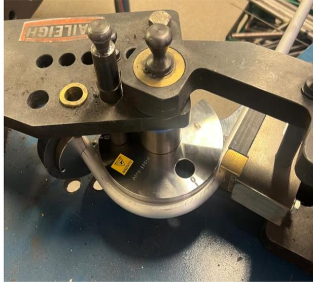
**Figure 4 Image of test piece of material in the tube bender.**
