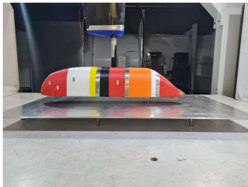
**Figure 7** : The 3D printed bodywork with strings attached in the wind tunnel experiment.
