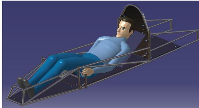
**Figure 14 Complete Chassis CAD Design with driver model.**
