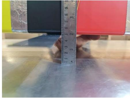
**Figure 6** The ground clearance setup during the wind tunnel experiment.
