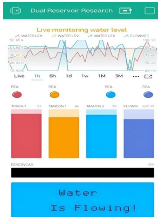
Figure 9. Blynk application display for 3 ultrasonic sensors and 1 flowmeter sensor
