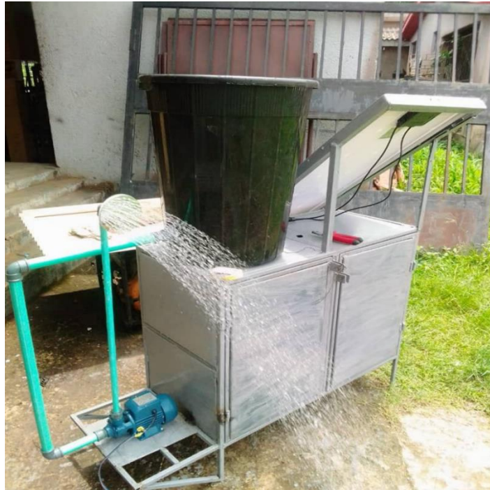
Fig.3 Diagram of the fabricated Solar Timer Pump System
