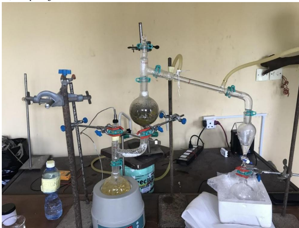
Fig. 2 Indirect steam distillation apparatus.
