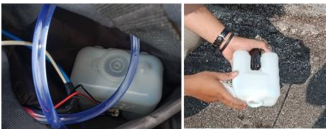
Figure 8. Installation of a water tank in a rucksack
