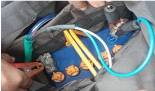
Figure 7. Installing the battery in the rucksack
