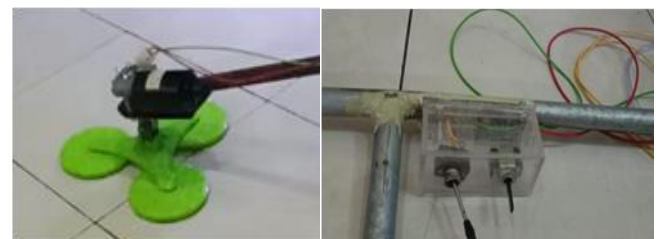
Figure 6. The rotary mop, cable, and hose system are assembled into a unit
