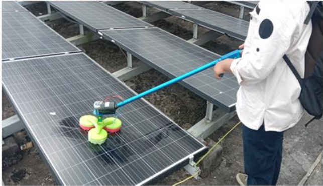
Figure 14. Prototype performance testing for wet cleaning method
