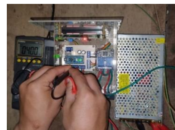
Figure 6. Testing the voltage divider circuit
