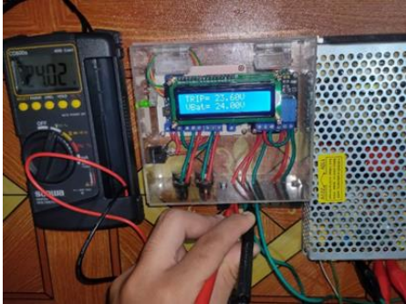
Figure 8. Testing voltage value readings with a 24V PSU
