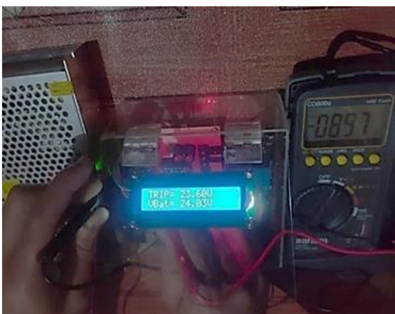
Figure 5. Testing the LM7809 IC as an Arduino Nano supply
