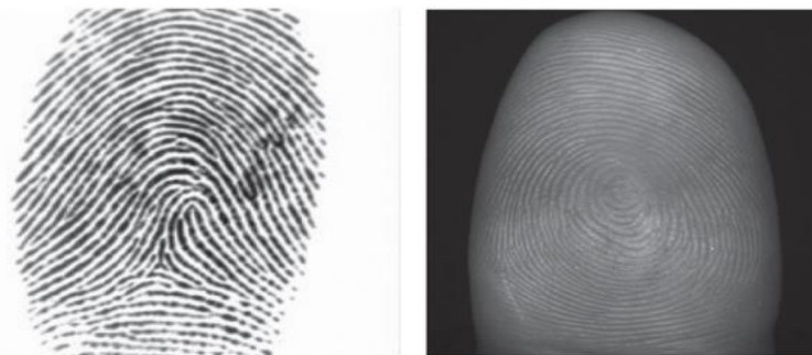
Figure 2. Contact fingerprint and contactless fingerprint comparison: (a) contact fingerprint image from FVC2002-DB1-A with image ID 1_2; (b) contactless fingerprint image from a benchmark set of data with image ID 1_1_1_0 [16].
