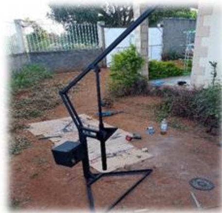
101: Base; 02: Barrel; 03: Heater; 04: Press support; 05:Hopper; 06: Control box; 07: Lever arm; 08: Injection cylinder.
