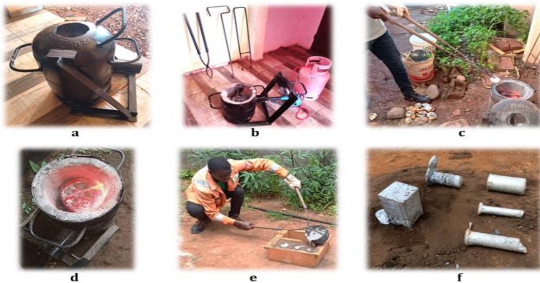
a - Furnace; b - Foundry elements; c - Supply of scrap cans in the crucible inside the furnace; d - Liquid aluminium in the heated crucible inside the furnace; e - Sand casting operation; f - Parts obtained.
