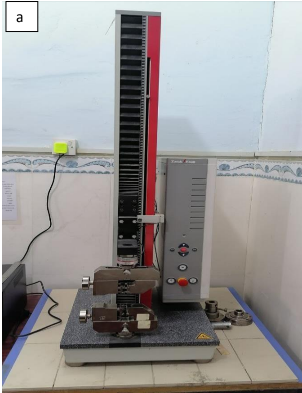
Figure 3: Equipment is used to assess the samples: (a) mechanical properties measuring device (Tensile), (b) The Hilmarc's Lee's Disc apparatus for thermal conductivity measurement.
