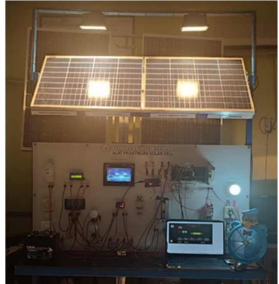
Figure 7. SCADA- Based Solar Panel Practicum Tool
