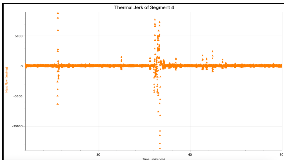
Figure 13. Thermal Jerk vs. Time graph for 8OCB for cooling at rate 5°C/min.
