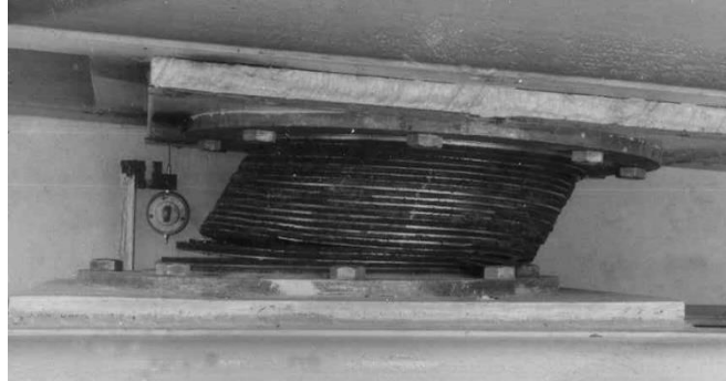
Figure 1. View of the first laminated rubber bearing manufactured in Armenia under testing
