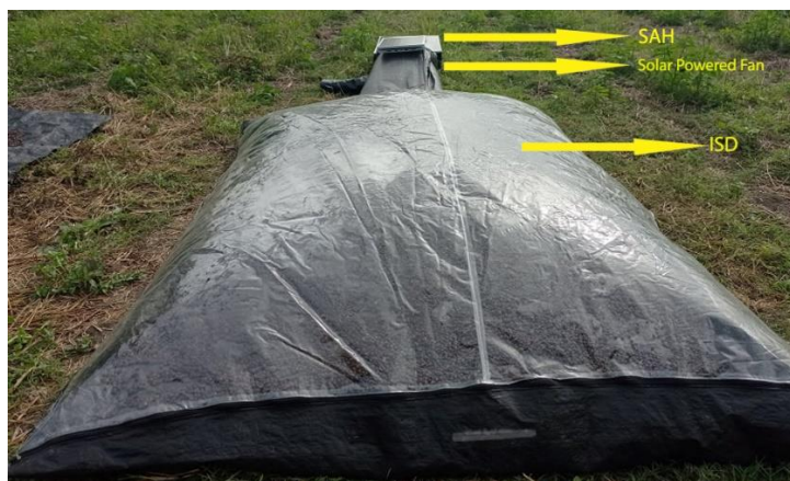
Figure 3. The ISD, SAH, and Solar powered fan
