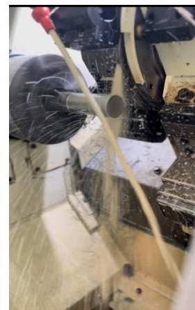
Figure 2. Wet cooling condition
