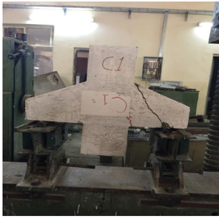
Figure 2: Failure Mode of Specimen (C1).
