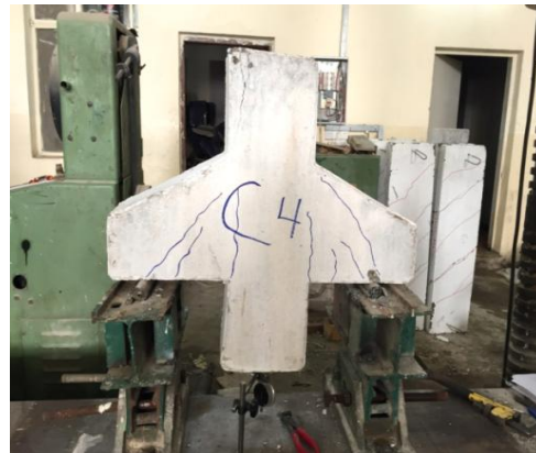
Figure 5: Failure Mode of Specimen (C4).
