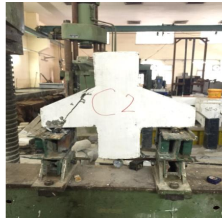
Figure 3: Failure Mode of Specimen (C2).
