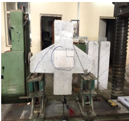
Figure 6: Failure Mode of Specimen (C5).
