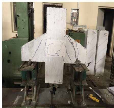
Figure 7: Failure Mode of Specimen (C6).
