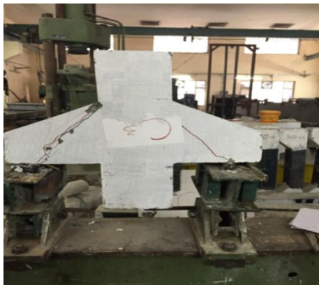
Figure 4: Failure Mode of Specimen (C3).
