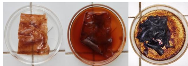
Figure 7. Uwi tuber plastic (left), plastic after being treated with EM4 (middle), plastic after 35 days degradation (right)
