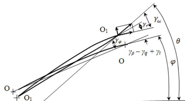
Fig. 1. Model for determining the departure angle
