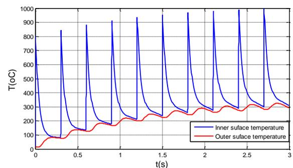
Fig. 6. Temperature graph of inner and outer walls of the artillery
