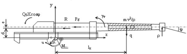
**Fig. 2. Diagram of forces acting on the range block when firing**
