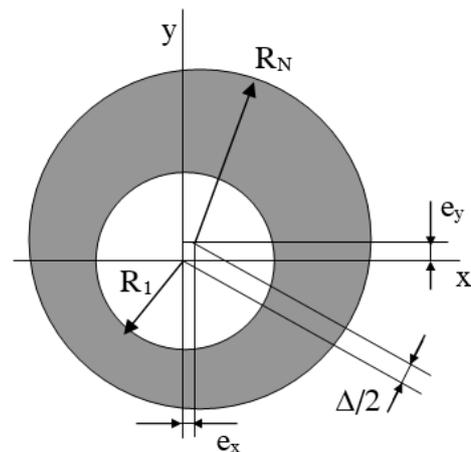
Fig. 3. Model for determining the departure angle when the barrel wall thickness is different
