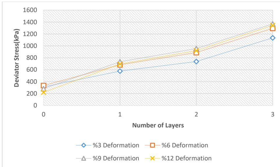
Fig. 18d. Under 200 Kpa Cell Pressure, Deviator Stress Values of Different Deformation Rounds
