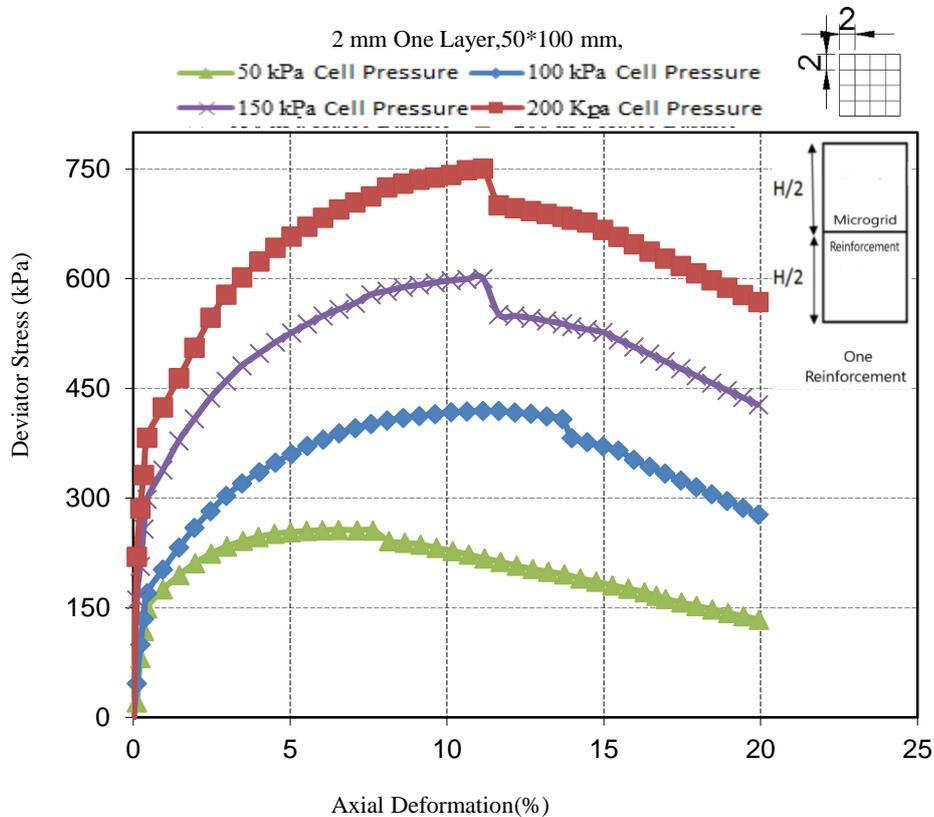
**Fig 9. One Layer Reinforced Sample Stress-Strain Curves**
