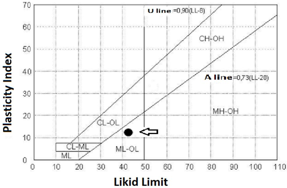
Fig 4. Casagrande Card of the Low Plasticity Silt
