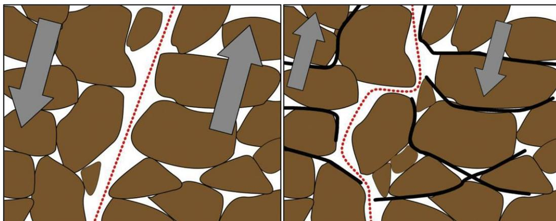
Fig.1. The Soil Matrix Reinforced with the Microgrids[3]
