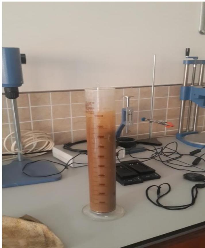
Fig 3. Hydrometer Experiment
