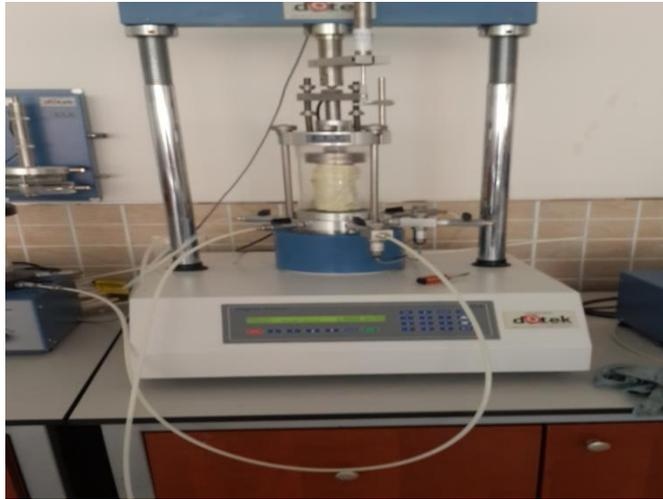
**Fig 7. Triaxial Compression Test Used for the Study**
