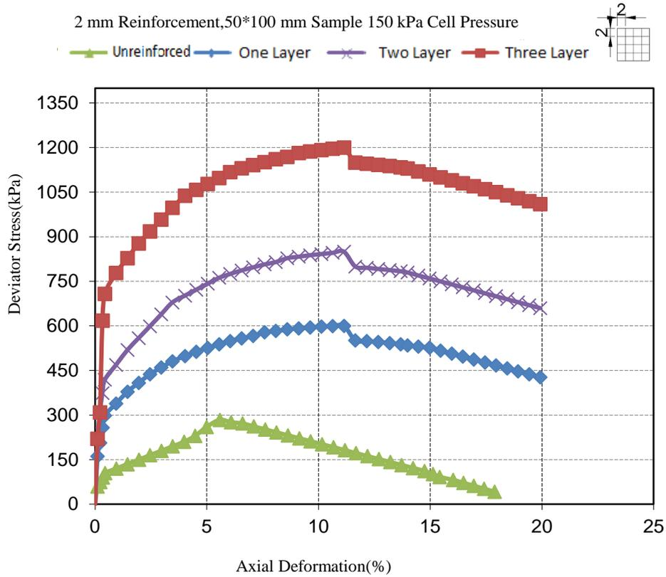
Fig. 14. 150 kPa Cell Pressured Stress- Strain Curves of Every Configuration
