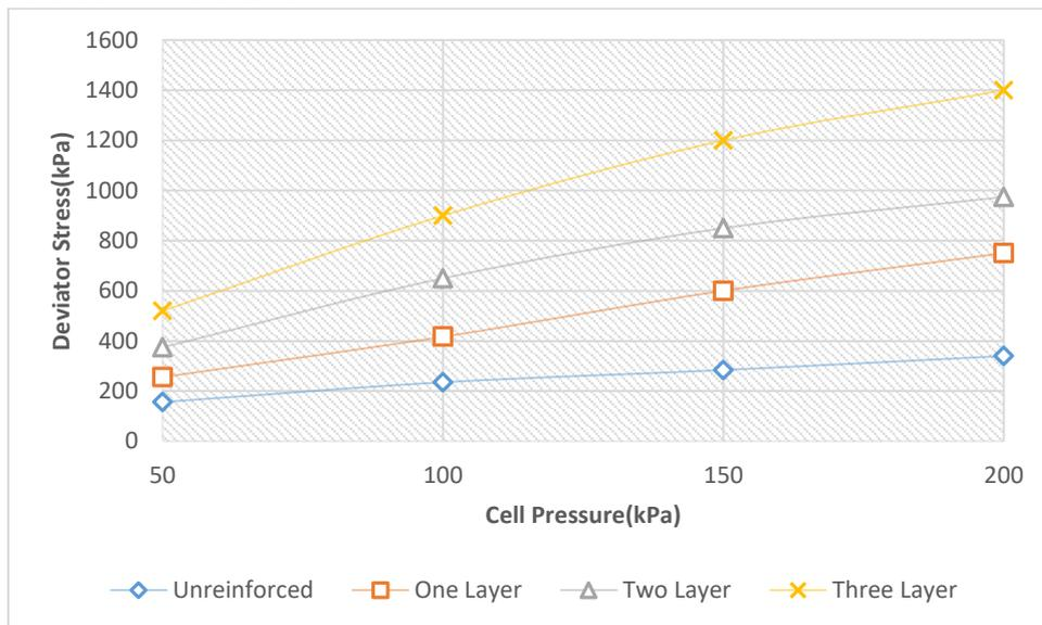
Fig. 17.Effect of Cell Pressure on Peak Deviator Stress of Soil
