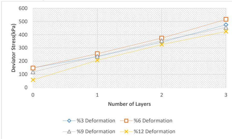
Fig. 18a. Under 50 Kpa Cell Pressure, Deviator Stress Values of Different Deformation Rounds
