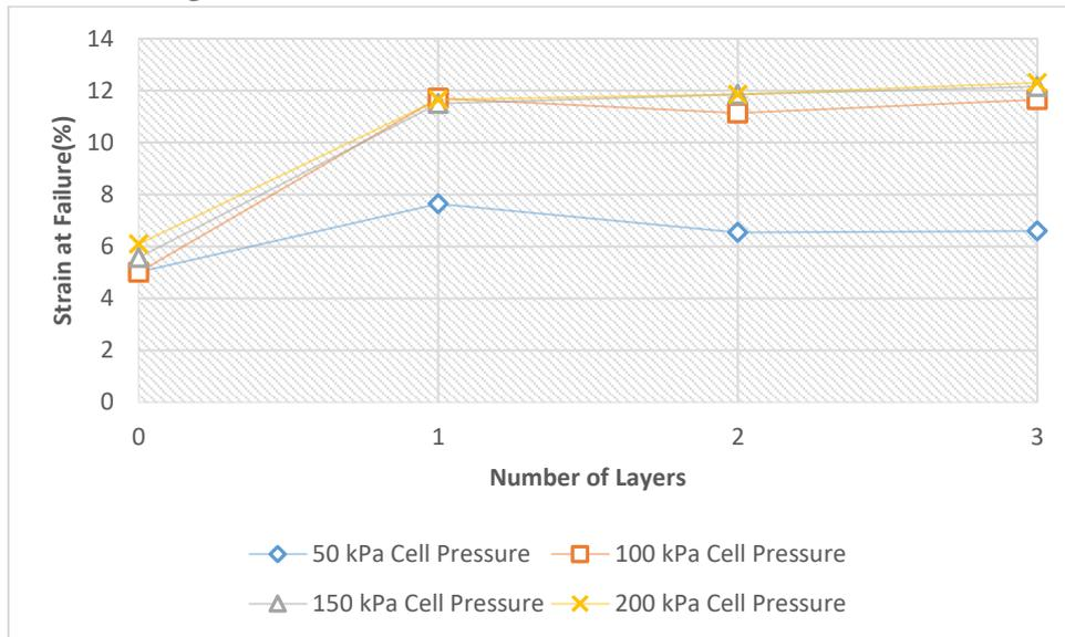
Fig. 19. Failure Strain Values of Every Layer Configuration Under Different Cell Pressures
