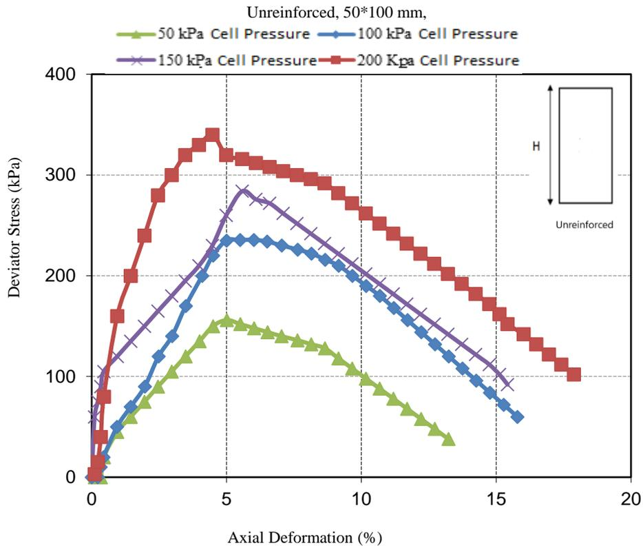
**Fig 8. Unreinforced Samples Stress-Strain Curves**
