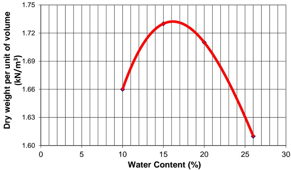
Fig 5. Proctor Curve of the Experimental Soil
