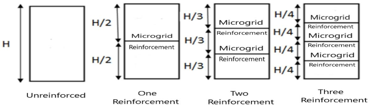
Fig 6. Reinforcement Configuration of the Experiments
