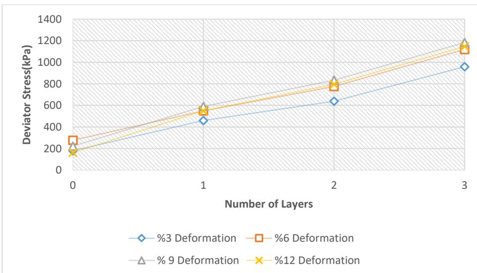
Fig. 18c. Under 150 Kpa Cell Pressure, Deviator Stress Values of Different Deformation Rounds
