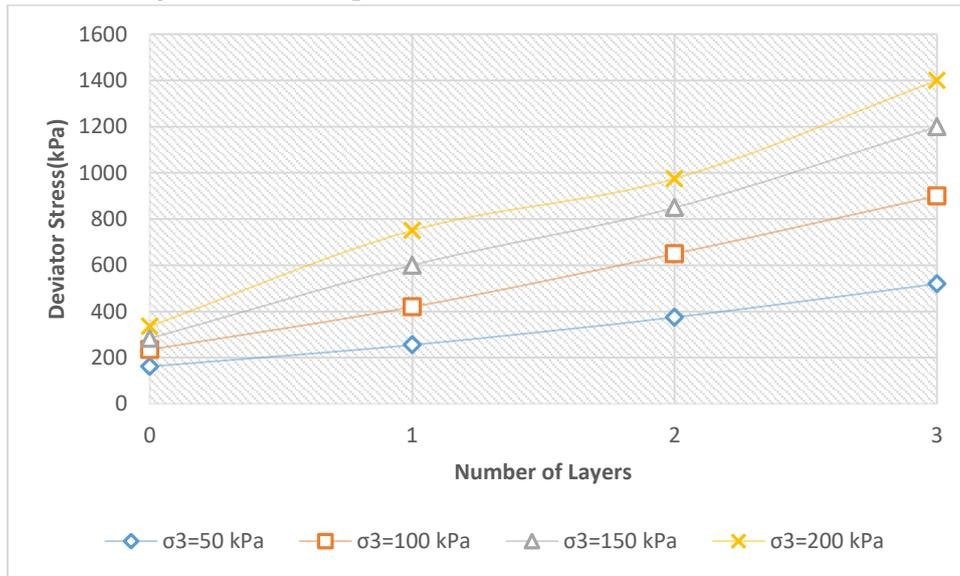
Fig. 16. Effect of Number of Layer Configuration
