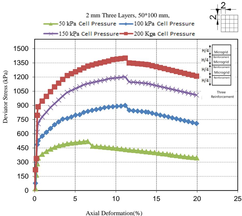
Fig. 11. Three Layered Reinforced Samples Stress- Strain Curves
