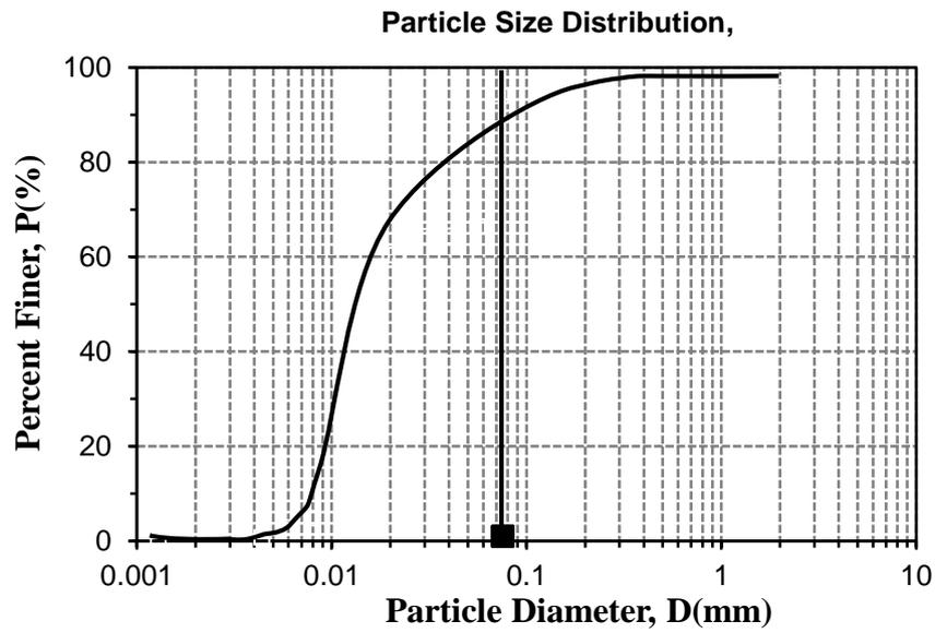
Fig 2. Particle Size Distribution of the Silty Soil
