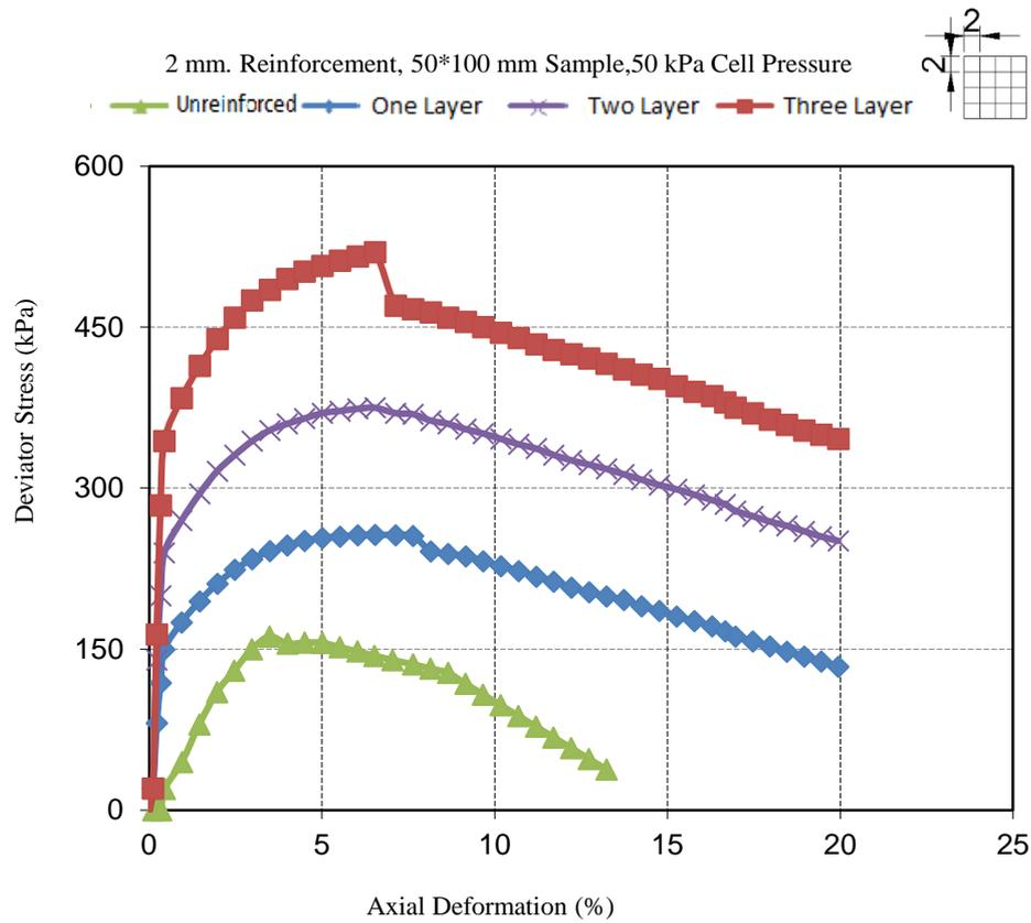
Fig. 12. 50 kPa Cell Pressured Stress- Strain Curves of Every Configuration
