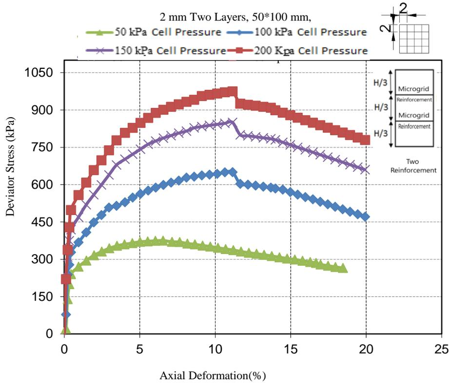
Fig. 10. Two Layered Reinforced Sample Stress-Strain Curves
