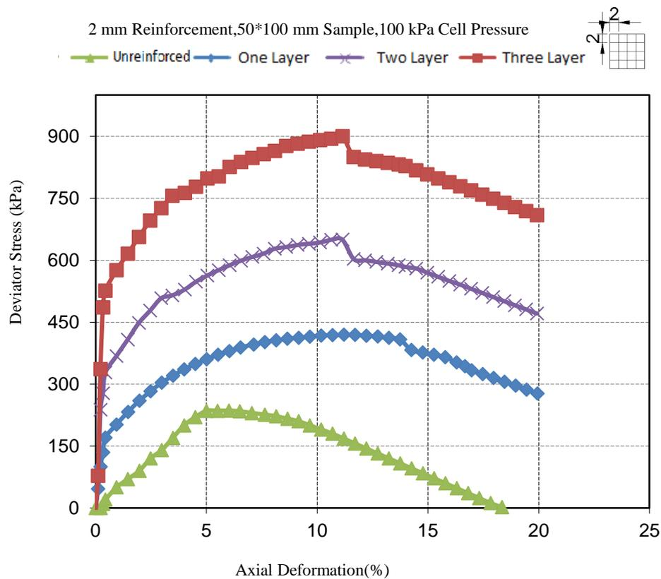
Fig. 13. 100 kPa Cell Pressured Stress- Strain Curves of Every Configuration
