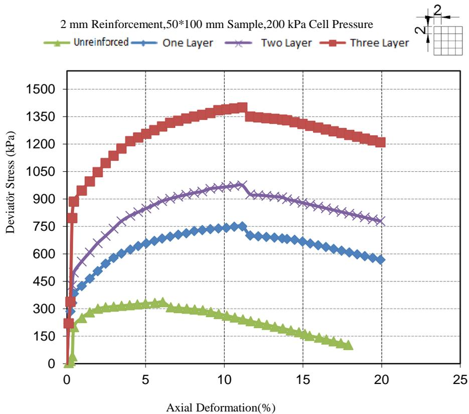
Fig. 15. 200 kPa Cell Pressured Stress- Strain Curves of Every Configuration
