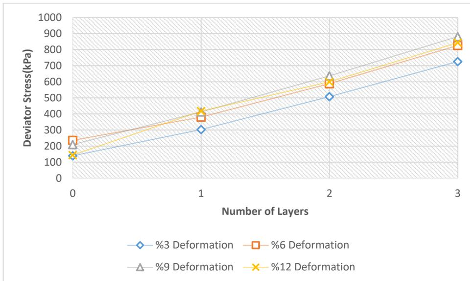
Fig. 18b. Under 100 Kpa Cell Pressure, Deviator Stress Values of Different Deformation Rounds
