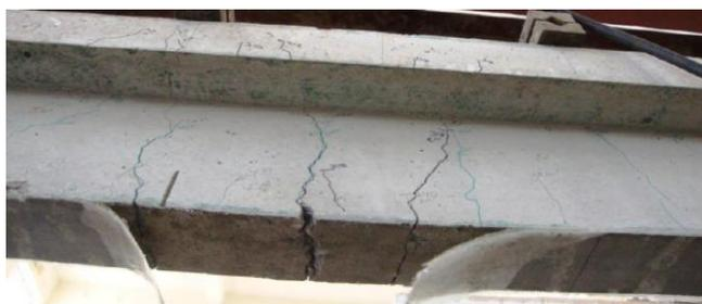
Figure 13: De-bonding of GFRP sheet from surface
