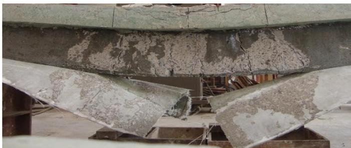
Figure 15: De-bonding of GFRP from web of Beam
