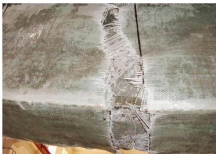
Figure 16: Failure of GFRP sheet
