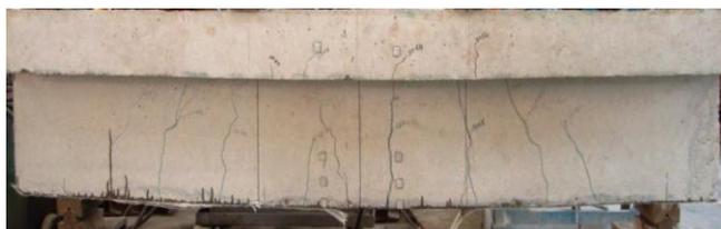
Figure 12: Picture of T-beam strengthened at the soffit
