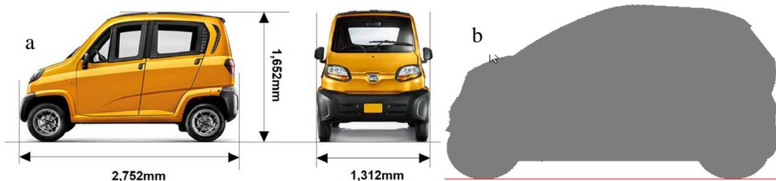
**Figure 1. Exterior overall dimensions (a) and CAD model (b) of BAJAJ QUTE**
