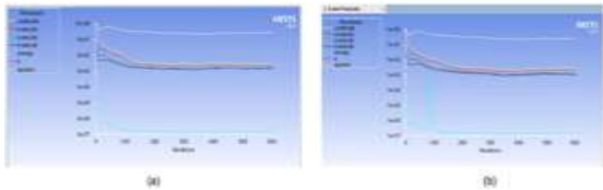
Fig 6: (a) and (b) Convergence of simulation (Baffle spacing of 120 mm and 240 mm).
