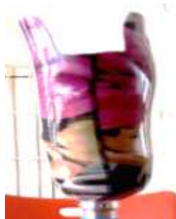
Figure 1.1: Transtibial prosthetic socket made from natural fibre
