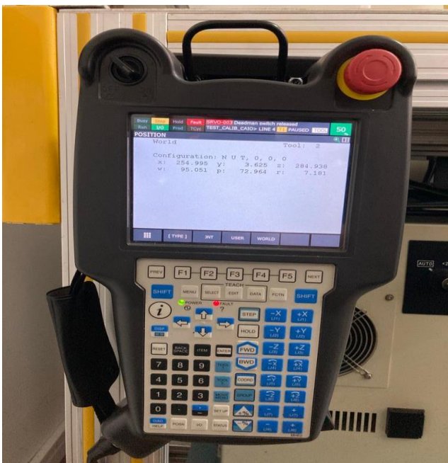
Figure 24. Result of positioning the robot in the "TP" teach pendant.
