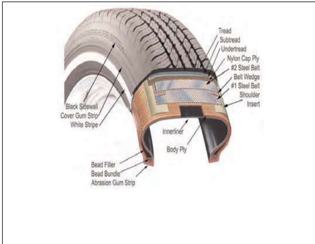
Fig. 5 Tire components. It is seriously past that the use of cables has spread in many areas and it is indispensable that a study should be made to compare some of the uses of cables, especially in bridges and tires.
