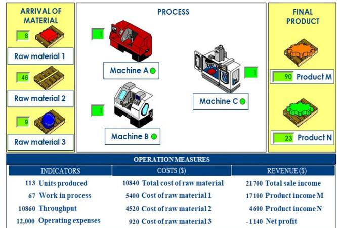
**Figure 3.** Representation of the current ProModel® system layout.
