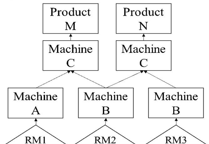
**Figure 2.** Operation diagram of the manufacturing system.
