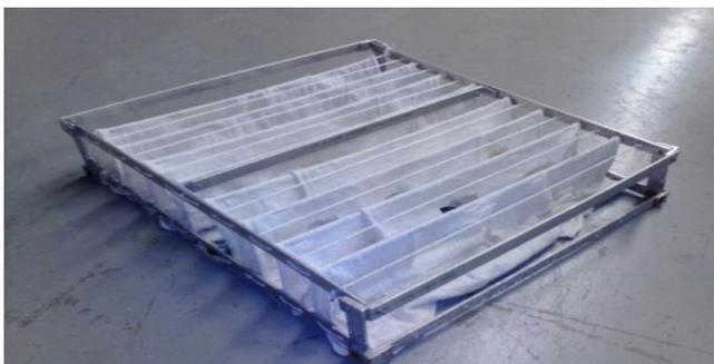
Fig. 2.Eight rows of the wick material used to increase the area of evaporating surface inside the basin of the still.
