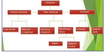
Fig. (1): A classification scheme for the various composite types [1].
