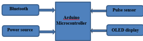
Figure 1: Block diagram for a RPO
