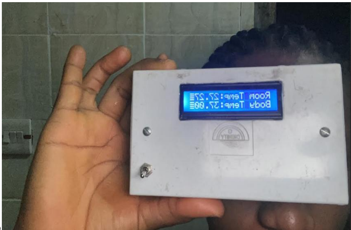
Figure 12a, b, & c: The device from when it is turned on to when it is placed over a forehead and reads both room temperature of 27.27°C and body temperature of 37.0°C
