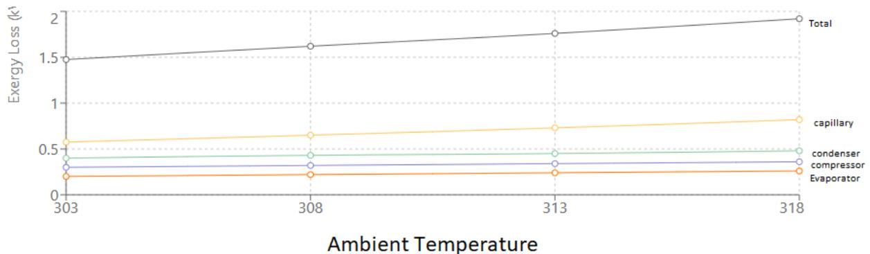
Fig. 4: Exergy losses (kW) vs. ambient temperature (K) for the four main devices and the total exergy loss.
