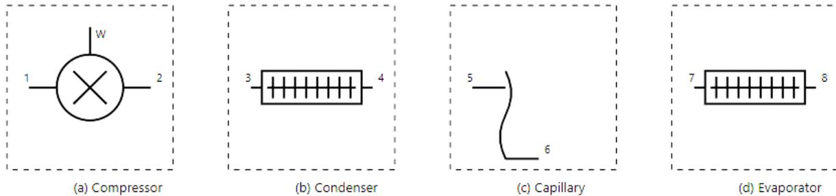
Fig. 3: Schemas of control volumes for the four main devices of a vapor compression refrigeration system:
