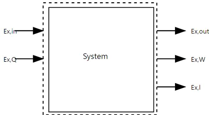
Fig. 2: The general exergy balance of a steady thermal system.
