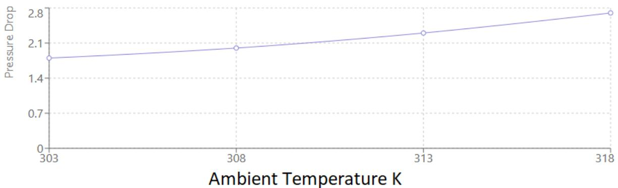
Fig. 5: Pressure drops (kPa) of the capillary during operation.
