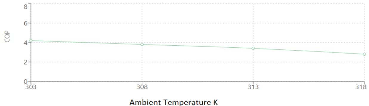
Fig. 6: COP of the refrigeration cycle vs. ambient temperature (K).
