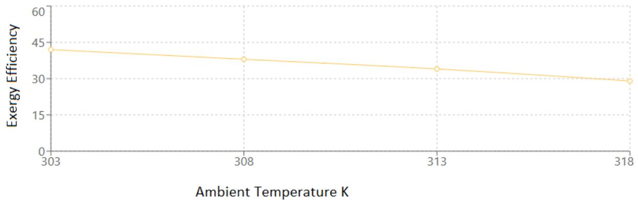
Fig. 8: Exergy efficiency vs. ambient temperature (K).
