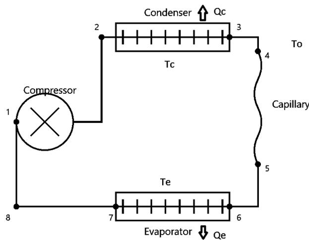
**Fig. 1: Schema of a basic vapor-refrigeration cycle**
