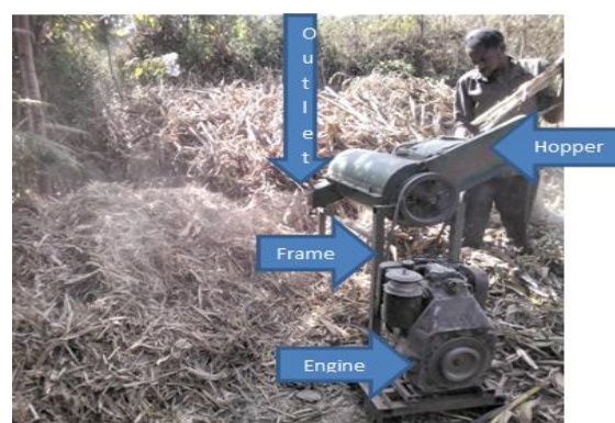
Figure 1b:- Animal feed chopper during field test
