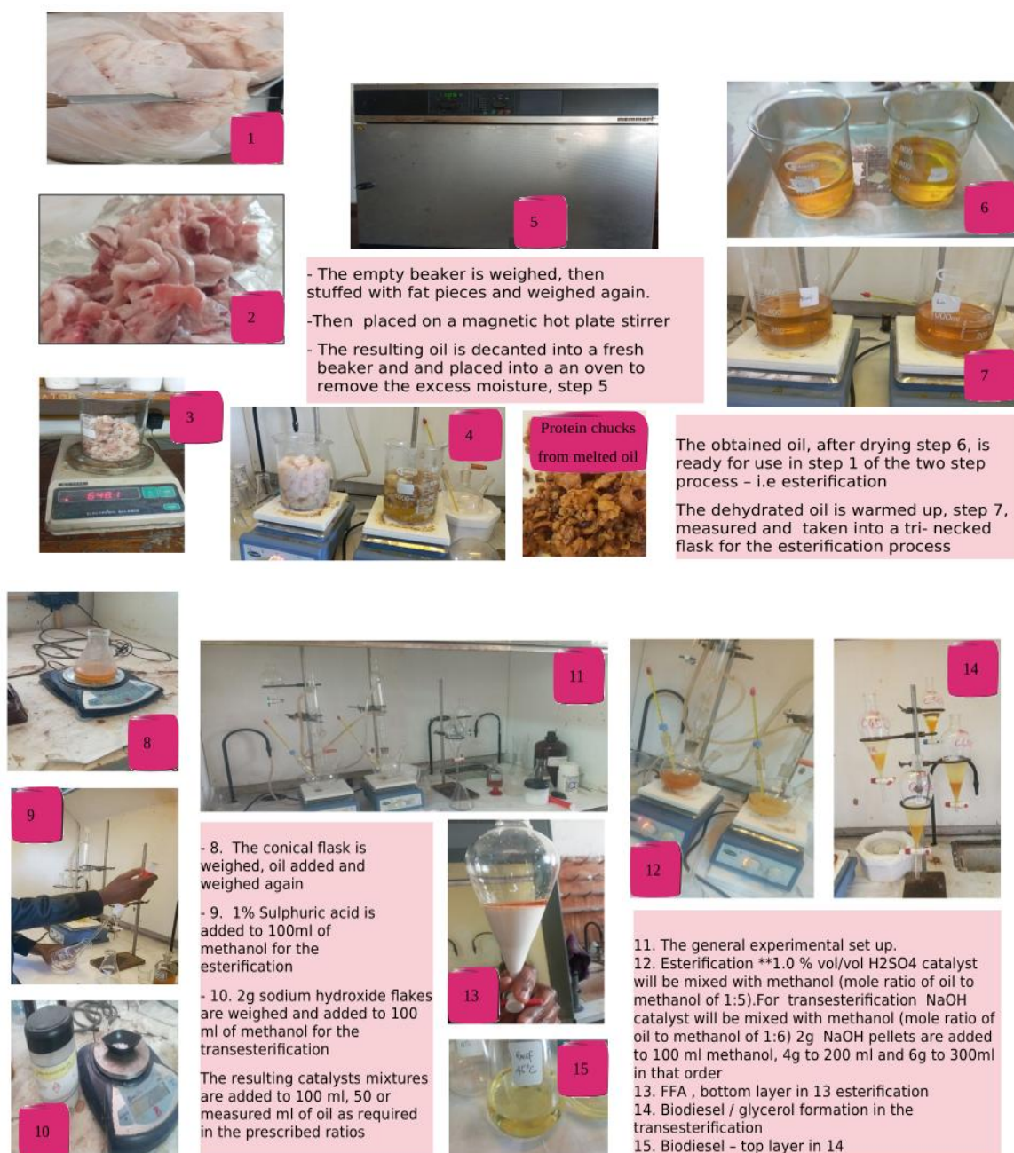
Fig 7. The modified two- step biodiesel synthesis process in pictures
