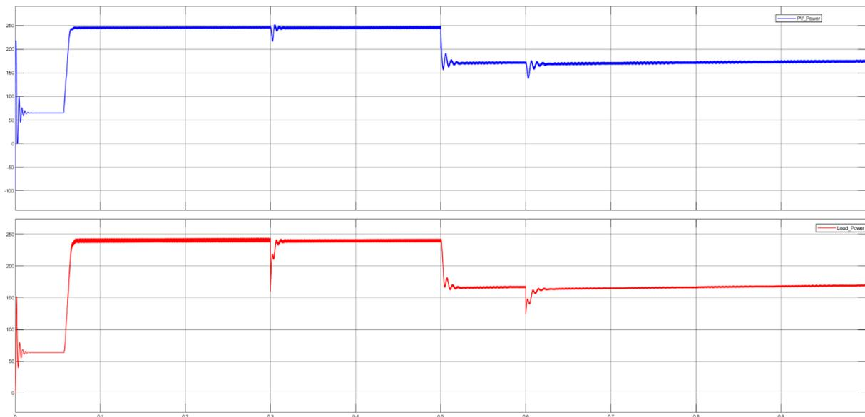
Figure 8. The output PV POWER under constant irradiance and variable temperature level.
