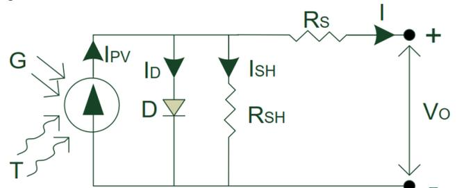
**Figure 1. Single diode equivalent circuit model of a photovoltaic cell.**
