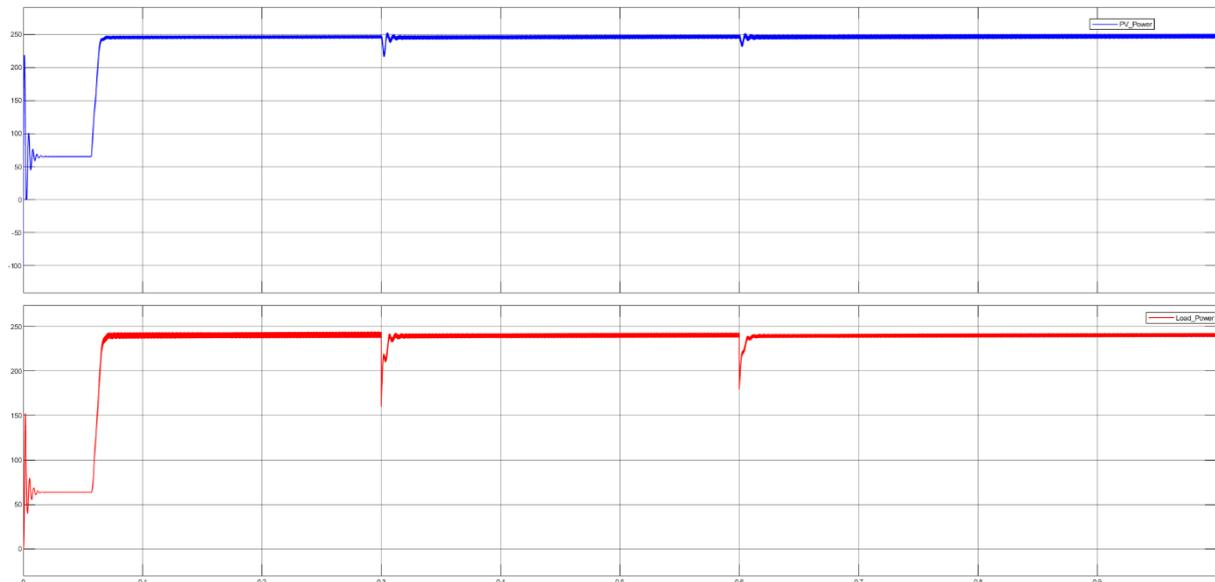
**Figure 6. The output PV POWER under constant irradiance and temperature.**
