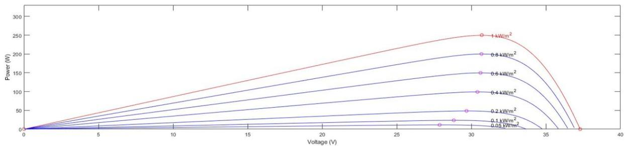
**Figure 2. Output power and voltage of the photovoltaic panel at constant temperature with varying solar radiation.**
