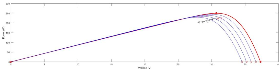
**Figure 3. Output power and voltage of the panel during constant solar radiation and various temperatures.**
