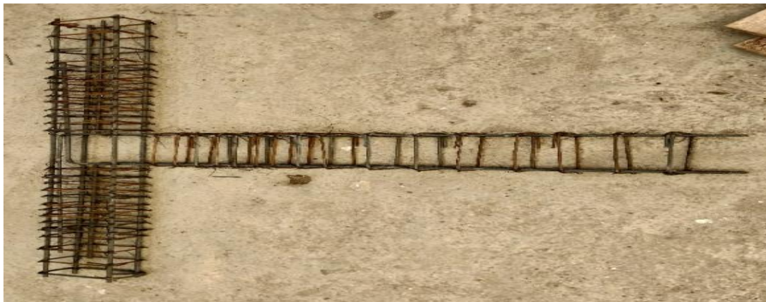
Fig No.3 Conventional Steel Reinforcement of Beam-Column
