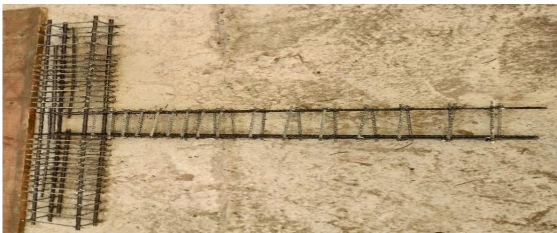
Fig No.4 Basalt Reinforcement of Beam-Column
