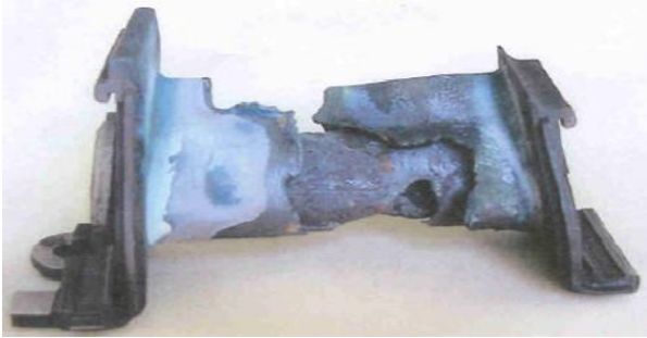
Plate 1: Overheated 1 st stage nozzle, up to complete melting.
