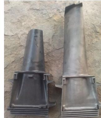
Plate 3: Gas Turbine Buckets
