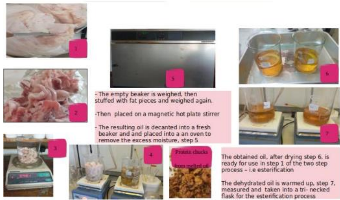
Fig 4a Oil extraction from fat
