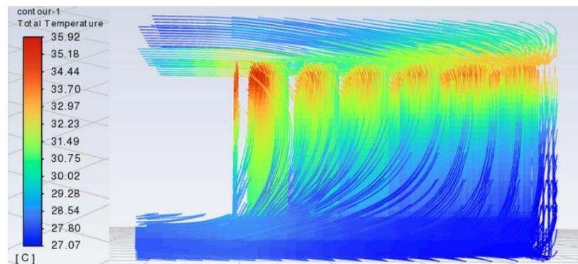
**Figure 13. Contour of the Temperature Distribution for the U-Channel Battery at  $Re = 15000$  under  $60^\circ\text{C}$  Operational Temperature**
