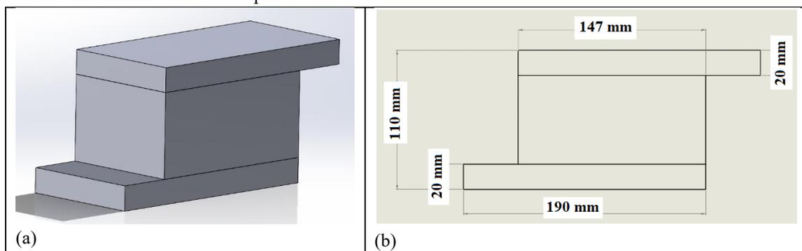
Figure 1. Z channel (a) General view, (b) Dimensioned version
