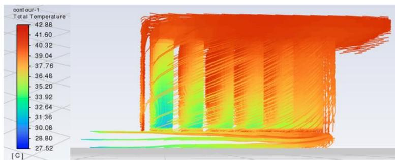
**Figure 8. Contour of the Temperature Distribution for the Z-Channel Battery at Re = 4000 under 60 °C Operational Temperature**
