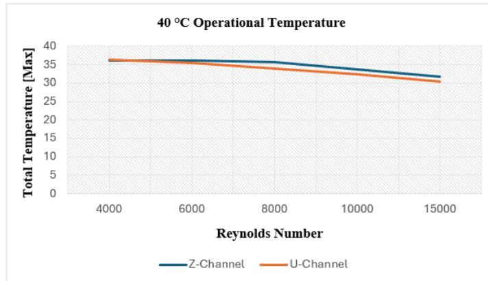
**Figure 21. Comparison of Maximum Temperature Values for Z-Channel and U-Channel Designs at  $40^\circ\text{C}$  Operational Temperature Across Various Reynolds Numbers**
