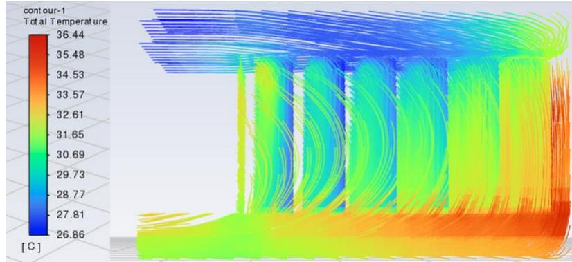
Figure 18. Contour of the Temperature Distribution for the U-Channel Battery at Re = 4000 under 40 °C Operational Temperature
