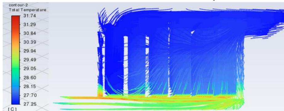
Figure 17. Contour of the Temperature Distribution for the Z-Channel Battery at Re = 15000 under 40 °C Operational Temperature
