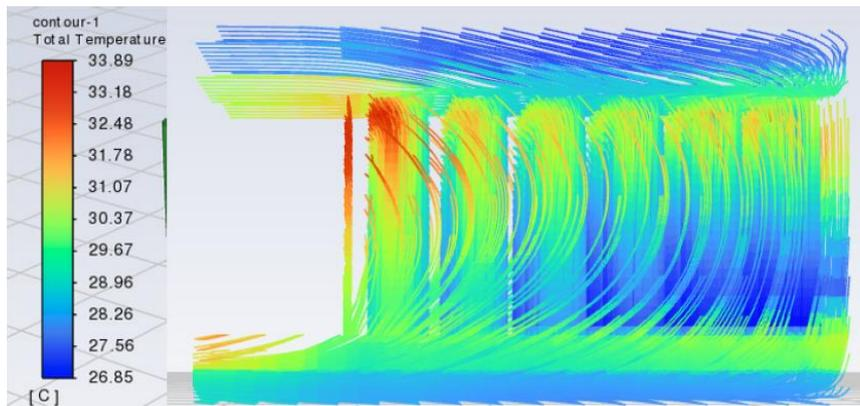
Figure 19. Contour of the Temperature Distribution for the U-Channel Battery at Re = 8000 under 40 °C Operational Temperature
