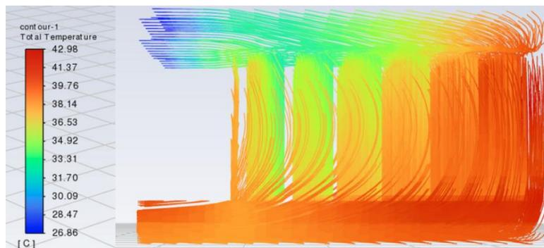
Figure 11. Contour of the Temperature Distribution for the U-Channel Battery at  $Re = 4000$  under  $60^\circ\text{C}$  Operational Temperature
