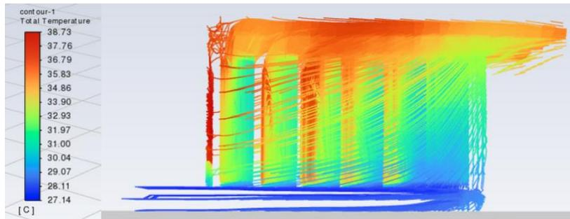
Figure 10. Contour of the Temperature Distribution for the Z-Channel Battery at  $Re = 15000$  under  $60^\circ\text{C}$  Operational Temperature
