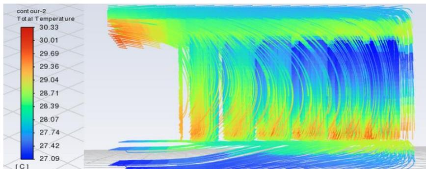
Figure 20. Contour of the Temperature Distribution for the U-Channel Battery at Re = 15000 under 40 °C Operational Temperature
