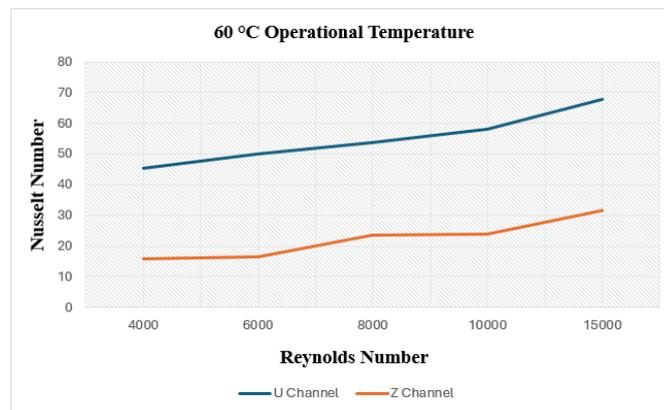
**Figure 22. Comparison of Nusselt Numbers for Z-Channel and U-Channel Designs at  $60^\circ\text{C}$  Operational Temperature Across Various Reynolds Numbers**
