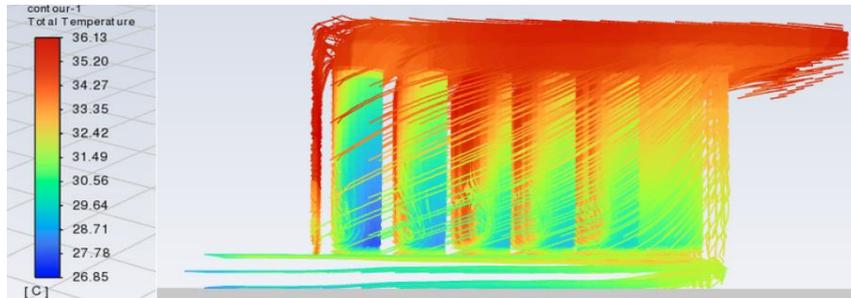
Figure 15. Contour of the Temperature Distribution for the Z-Channel Battery at Re = 4000 under 40 °C Operational Temperature
