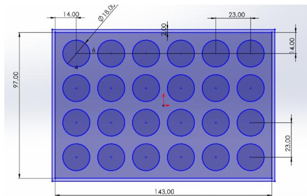
Figure 3. The positions of nickel-based cathode materials within the battery
