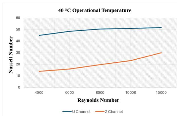
**Figure 23. Comparison of Nusselt Numbers for Z-Channel and U-Channel Designs at  $40^\circ\text{C}$  Operational Temperature Across Various Reynolds Numbers**
