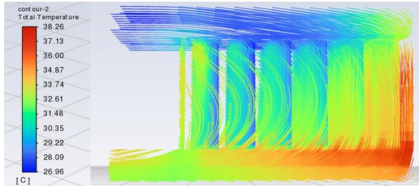
**Figure 12. Contour of the Temperature Distribution for the U-Channel Battery at  $Re = 8000$  under  $60^\circ\text{C}$  Operational Temperature**
