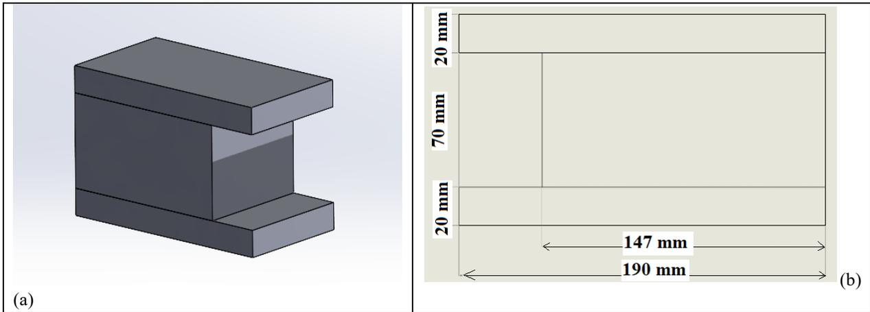
Figure 2. U channel (a) General view, (b) Dimensioned version
