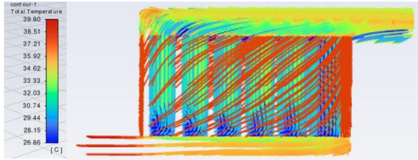
Figure 9. Contour of the Temperature Distribution for the Z-Channel Battery at  $Re = 8000$  under  $60^\circ\text{C}$  Operational Temperature
