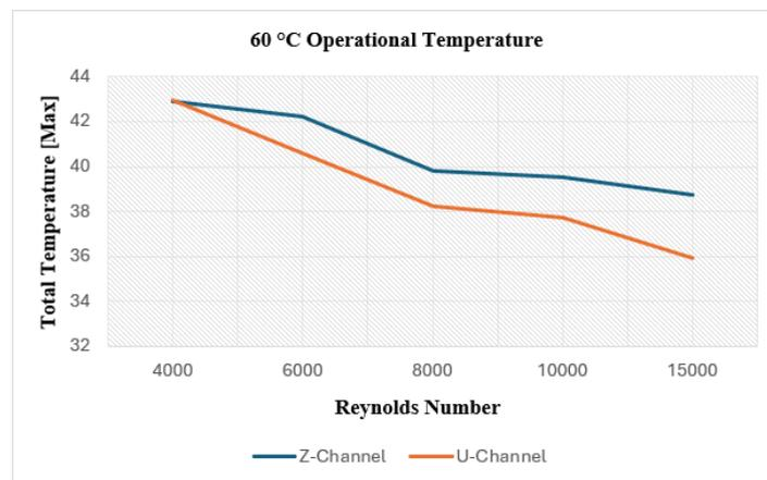
**Figure 14. Comparison of Maximum Temperature Values for Z-Channel and U-Channel Designs at  $60^\circ\text{C}$  Operational Temperature Across Various Reynolds Numbers**
