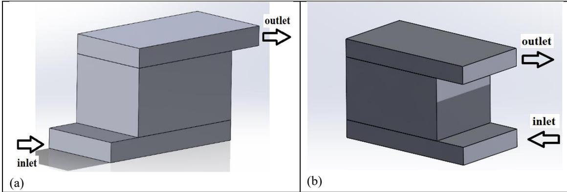
**Figure 7. Boundary conditions of li-ion battery (a) Z-channel, (b) U-channel**
