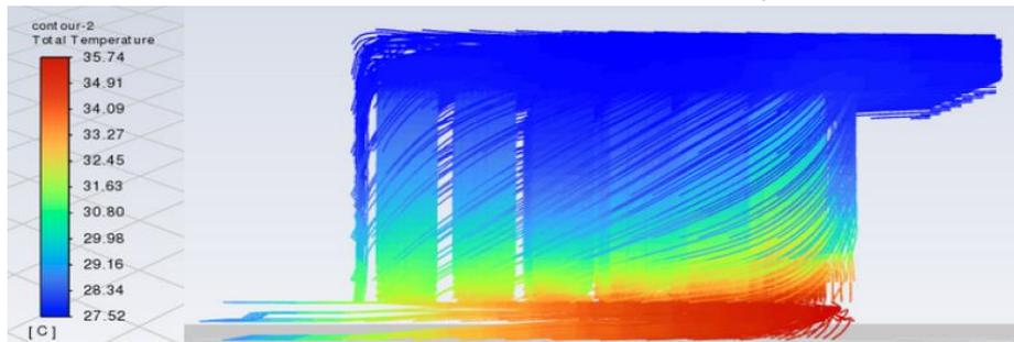
Figure 16. Contour of the Temperature Distribution for the Z-Channel Battery at Re = 8000 under 40 °C Operational Temperature
