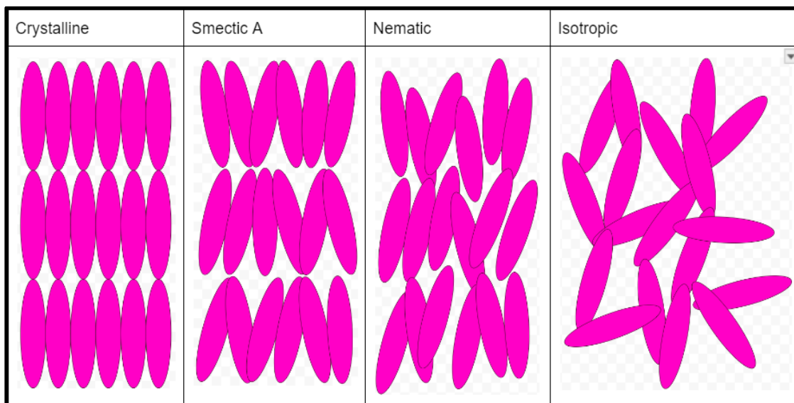
Figure 4: Molecular arrangement of 8CB liquid crystal showing mesophases. From left to right, it shows Crystalline, Smectic A, Nematic, and Isotropic. [15]
