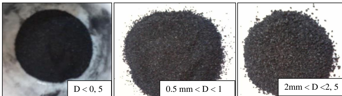
Figure 3: Date pits crushed and carbonized.(D= diameters)
