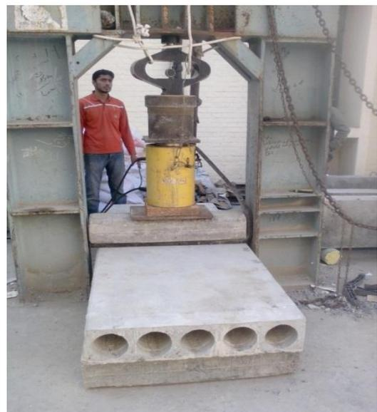
Figure 3: Testing arrangements for slabs in flexural loading
