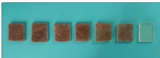
Figure 4: Samples for Archimedes density and Vickers hardness test.
