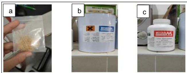
Figure 1: Materials used in sample fabrication a) Corn silk fibre, b) Epoxy type- MIRACAST 1517 (A), c) Hardener type- MIRACAST 1517 (B)
